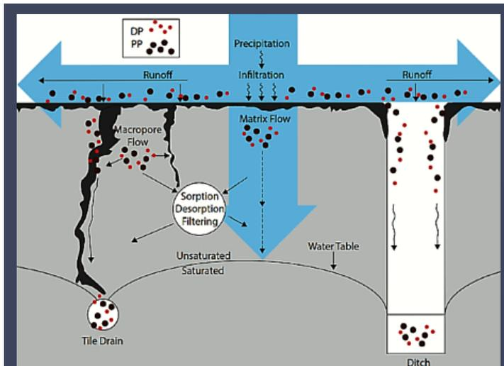
Figure 1. Flow diagram of water and P partitioning between surface runoff and infiltration and the partitioning of infiltration between macropore and matrix flow. DP, dissolved P; PP, particulate P. (Source: Radcliffe, et al. 2015)
